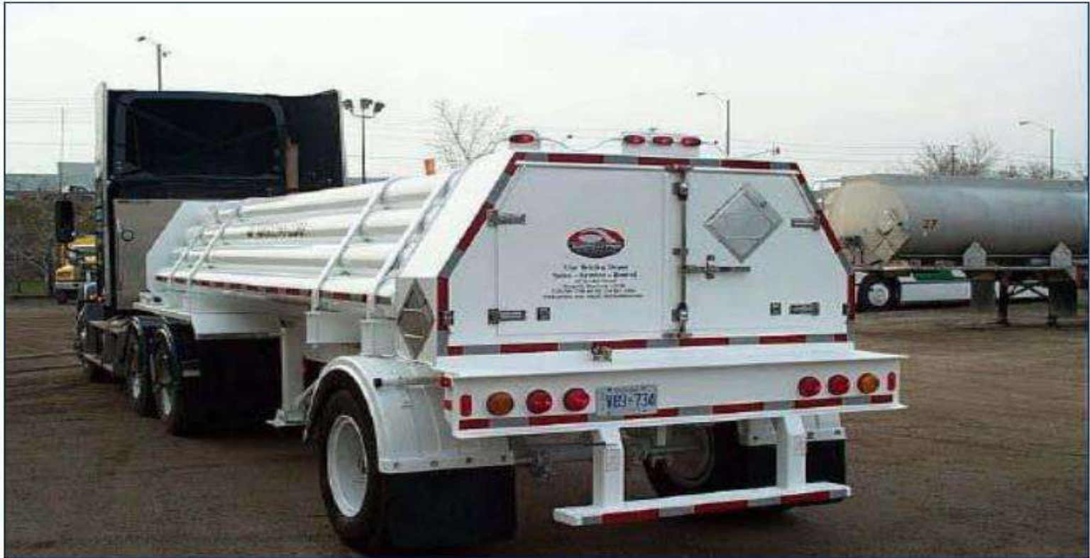
Figure 9: Compressed Hydrogen Gas Tube Trailer – 30 Cylinders and 43,260 SCF (105 kg) Capacity
