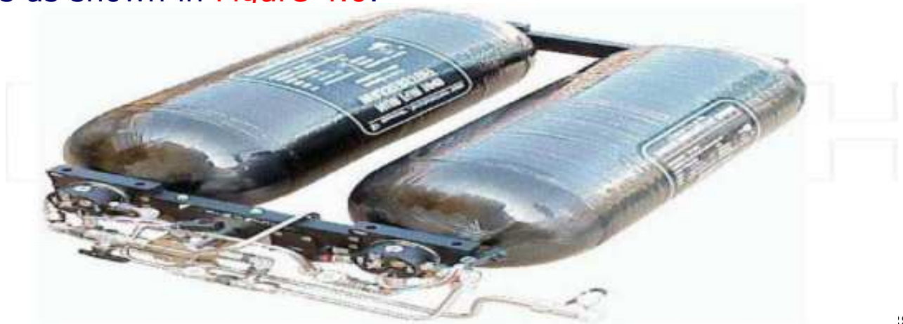
Figure 4. Hydrogen storage in tanks presently used in hydrogen-powered vehicles
