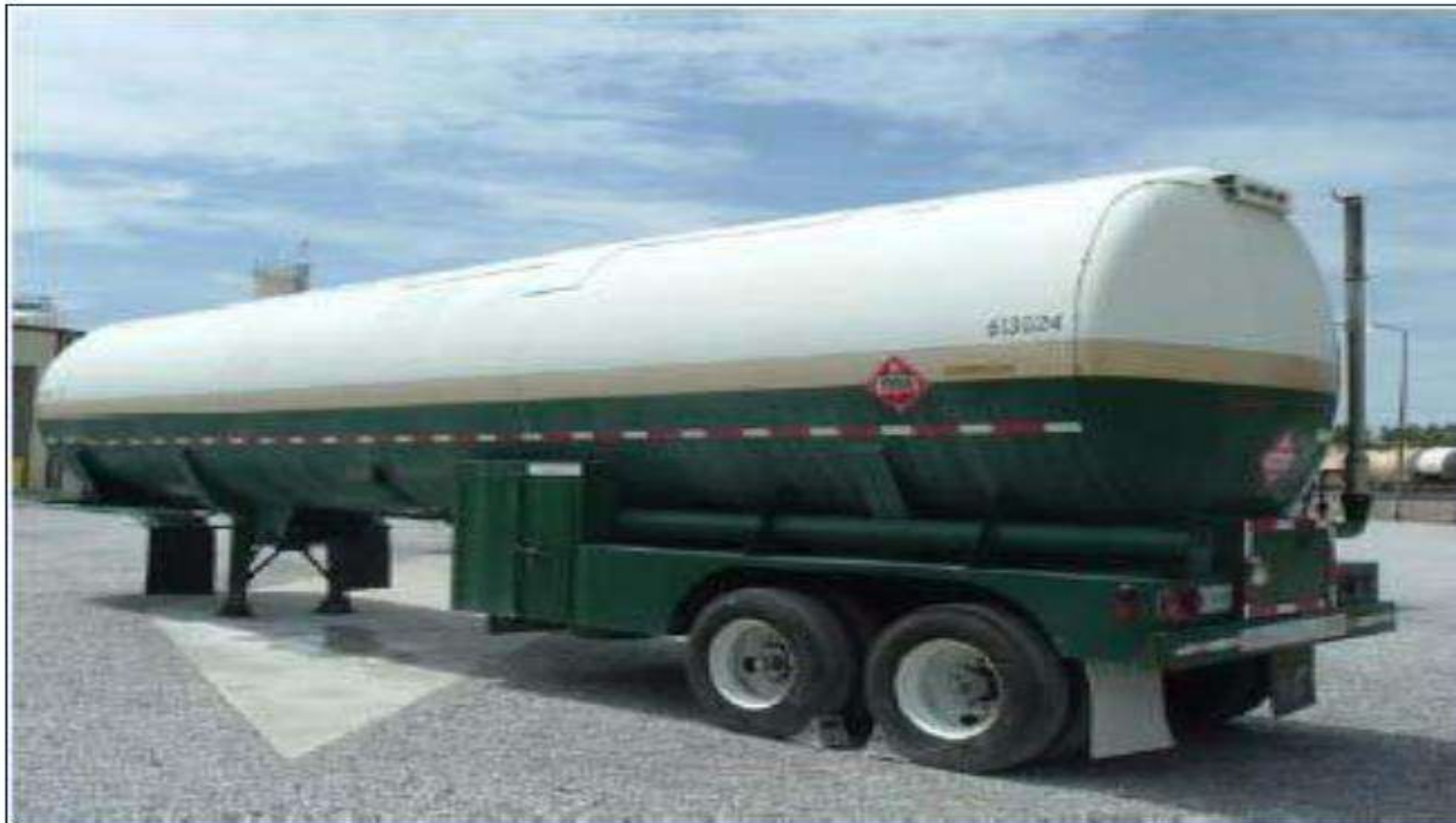
Figure 10: Cryogenic Liquid Hydrogen Trailer – 13,000 gallon (3,500 kg) capacity
