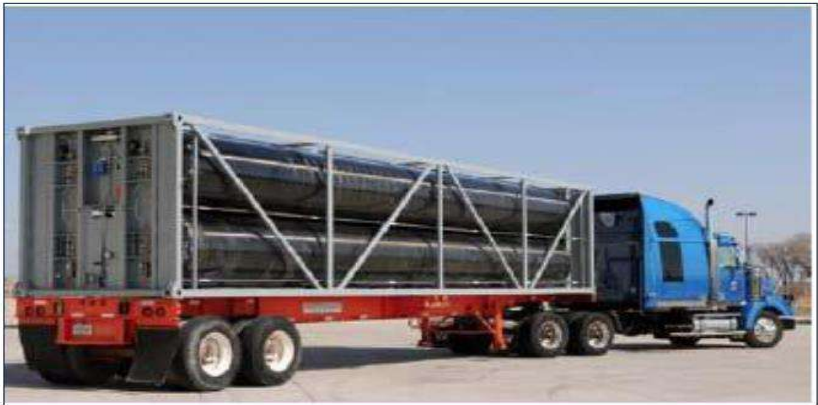
Figure 11: Next Generation Hydrogen Delivery System Undergoing Testing – 3,600 psi ISO Container for 600 kg of Transport Storage
